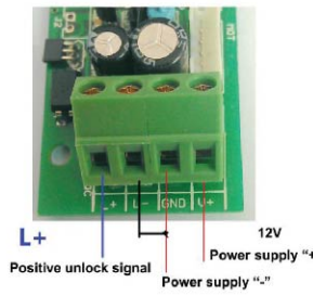
The positive unlock wiring diagram
